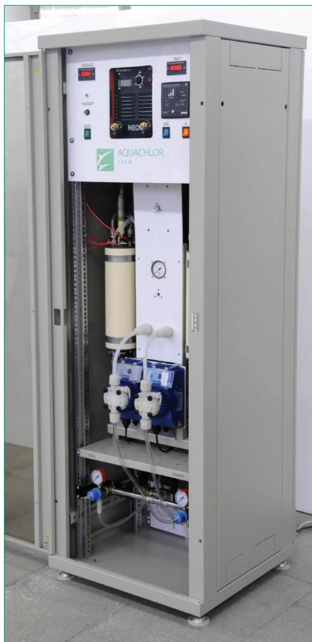
*Fig. 5.6. 6. AQUACHLOR-500M device with MB-26-100 cells operating in self-cleaning mode. Designed in 2011.*
