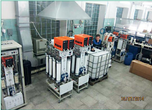
**Fig. 6.1.2.** *AQUACHLOR-1500M devices with a chlorine capacity of 1.5 kg per hour with MB-26D modular electrochemical elements in a dielectric body. The AQUACHLOR-1500M device contains 8 MB-26 elements of model 28600MIP4-05. Electric power consumption is 7.0 kW, weight 600 kg.*
