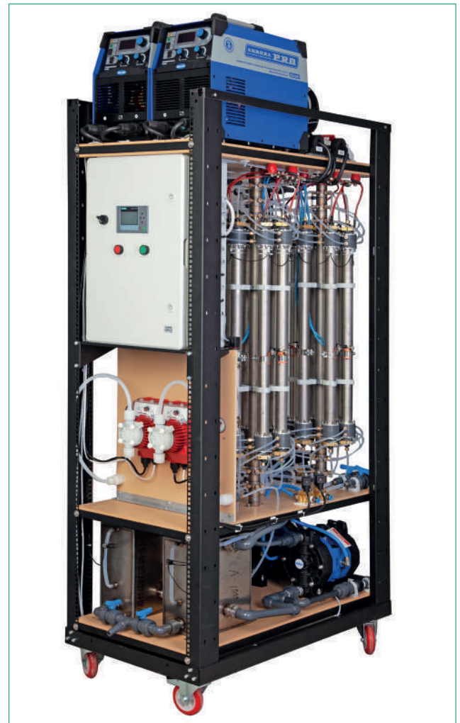
Fig. 6.2.6. AQUATRON-15-1500E device. The reactor of the device is made of twelve flow-through electrochemical modular elements MB-26T of a new generation with the use of ultrafiltration diaphragms made of chemically pure alumina in the alpha form.
