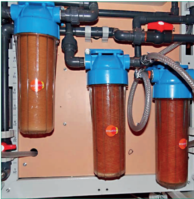
Fig. 6.2.10. Appearance of ten-micron filters of the EMERALD-UNIVERSAL-500 experimental device after 4 hours of operation on fresh artesian water with a content of ferrous iron ions of about 3 mg/l. From left to right, filters numbered F1, F2, and F3 shown in Fig. 6.2.7 and 6.2.8.
