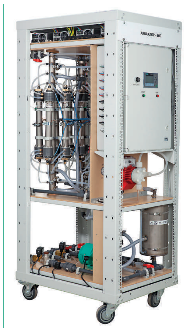
Fig. 6.3.15. STEL-ANK-SUPER-1000 (AQUACHLOR-600) Device. Vitold Bakhir Electrochemical Systems and Technologies Institute. Moscow, 2019.
