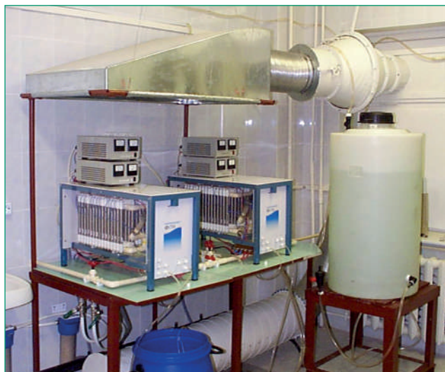
Fig. 6.3.7. STEL devices (NPO EKРАН) for the production of Anolyte ANK (500 l/h) in the «Anolyte» room Moscow City Hospital №915, Moscow, 1999.
