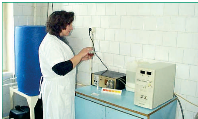
Fig. 6.4.1. STEL-10N-120-01 device (model 80) with a capacity of 80 l/h for anolyte ANK. City Clinical Hospital No. 52, 1999.
